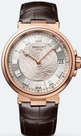
Case in 18-carat rose gold with fluted caseband. Sapphire-crystal caseback. 40 mm diameter. Silvered gold dial, engine-turned. Facetted Breguet hands in gold with luminescent material. Central seconds hand. Date at 3 o'clock. Mechanical self-winding movement, Cal. 777A, 55-hour power reserve. Inverted in-line lever escapement with silicon horns. Balance spring in silicon. Frequency 4 Hz. Screw-locked crown. Available on a rubber strap, ref. 5517BR/12/5ZU.
