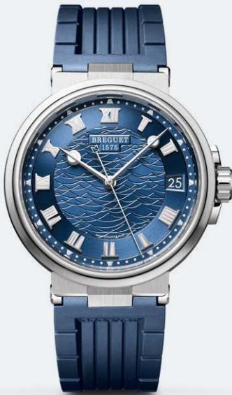
Case in 18-carat white gold with fluted caseband. Sapphire-crystal caseback. 40 mm diameter. Blue dial in gold, engine-turned. Facetted Breguet hands in gold with luminescent material. Central seconds hand. Date at 3 o'clock. Mechanical self-winding movement, Cal. 777A. 55-hour power reserve. Inverted in-line lever escapement with silicon horns. Balance spring in silicon. Frequency 4Hz. Screw-locked crown. Available on a leather strap, ref. 5517BB/Y2/9ZU.
