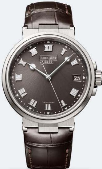
Case in titanium with fluted caseband. Sapphire-crystal caseback. 40 mm diameter. Sunburst slate grey dial in gold. Facetted Breguet hands in gold with luminescent material. Central seconds hand. Date at 3 o'clock. Mechanical self-winding movement, Cal. 777A. 55-hour power reserve. Inverted in-line lever escapement with silicon horns. Balance spring in silicon. Frequency 4 Hz. Screw-locked crown. Available on a rubber strap, ref. 5517TI/G2/5ZU.
